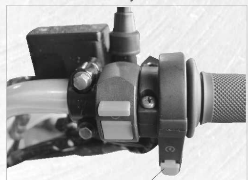
electrical start button
