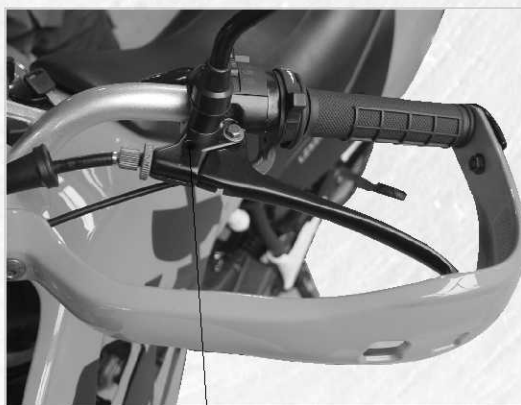
electrical start control switch
