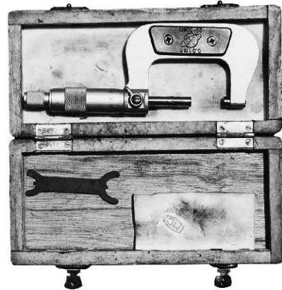
Micrometer: to measure the dimensions of piston, piston pin, etc.
